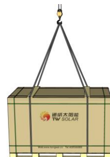
Figure 6 Schematic diagram of Module lifting
