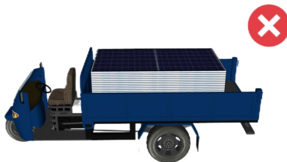
Figure 10 Do not use a tricycle to transport the Module
