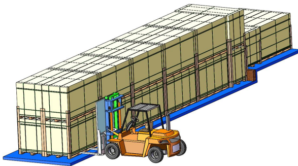
Short-side vertical package and U-shape package unloading with forklift
